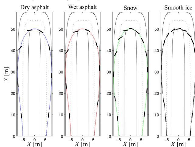
**Figure 2:** Trajectory in the XY-plane for the different road surfaces. The black rectangles indicate the position and direction of the vehicle each second [5].
