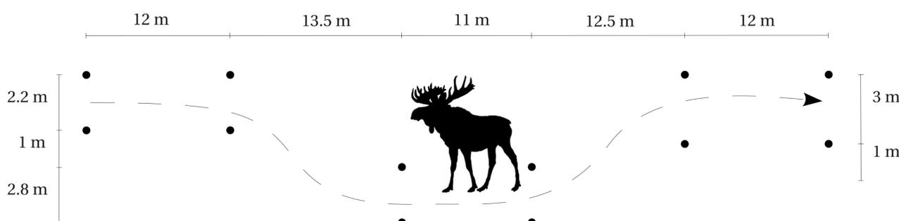
**Figure 3:** A sketch over the double lane-change maneuver, based on [3].
