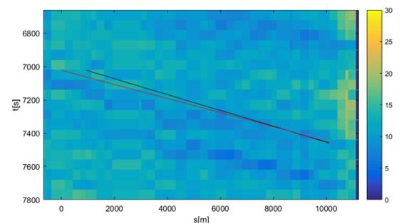
**Figure 2:** Traffic density and truck trajectories.
