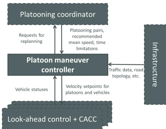
**Figure 1:** Preliminary architecture - Between the centralized platooning coordinator and vehicle and platoon controllers.
