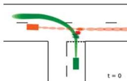
Figure 2: Screenshot from the visualisation of the simulation environment, illustrating the probabilistic prediction of the adjacent (red) vehicle as well as the possible collision points
