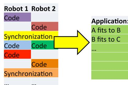
Today, industrial robots are programmed line-by-line for each robot, and are manually synchronized. The goal is to move into a higher level of abstraction, by declaring temporal, logical and geometrical rules of the robots and the application, as well as goals of the latter. A throughput optimal robot program is output, with provable robustness.
