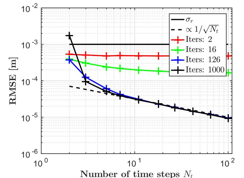
**Figure 4:** Monte Carlo Simulations for the error of positions for different amount of iterations in the alternating optimization scheme. More recorded time-steps yields better accuracy of the estimated  $r_k$ .  $\sigma_r$  is the standard deviation of the positions  $r_k$ .
