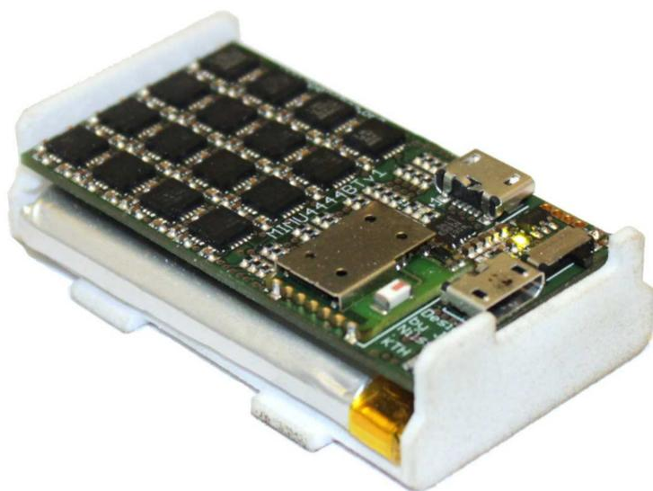
**Figure 1:** An in-house designed embedded system with an inertial sensor array. The array consists of 32 MPU9150 Invensense inertial sensor chipsets, each containing an accelerometer triad, a gyroscope triad, and a magnetometer triad. The device measures 53 mm x 33 mm.
