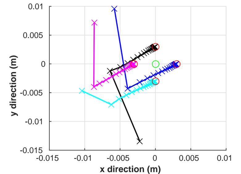
**Figure 3:** Convergence of the positions of 5 accelerometers in the  $xy$ -plane, the green circle is the reference accelerometer, and the red circles are the true positions.
