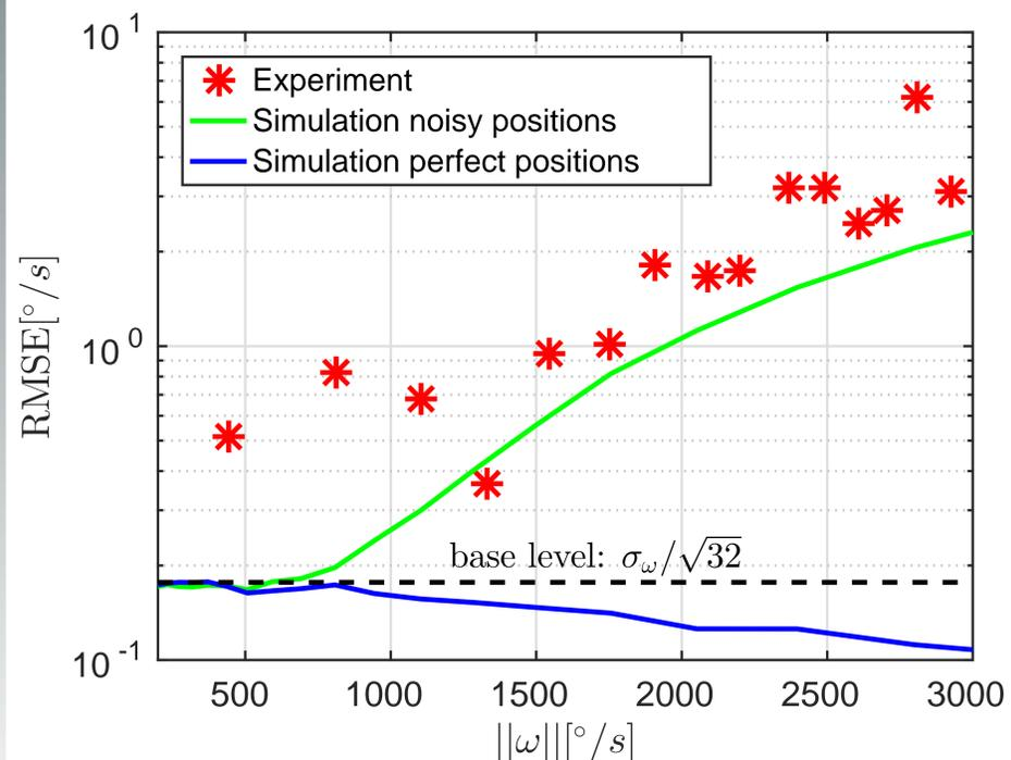
**Figure 2:** RMSE of experimental measurements, simulations with imperfect positions, and simulations with perfect positions.  $\sigma_\omega$  is the standard deviation of a single gyroscope.
