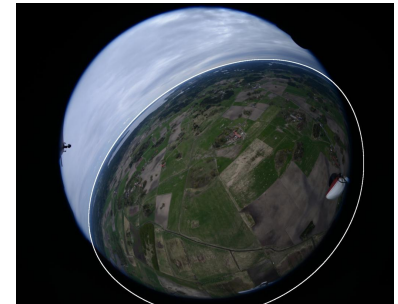
Detected horizon line for attitude estimation.
