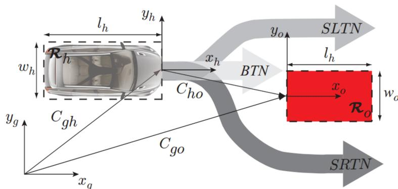
Figure 2: Possible avoidance maneuvers of an automated road vehicle. Figure taken from [2]
